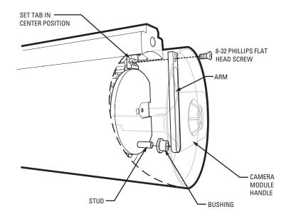
Figure 8. Install Wiper Arm
